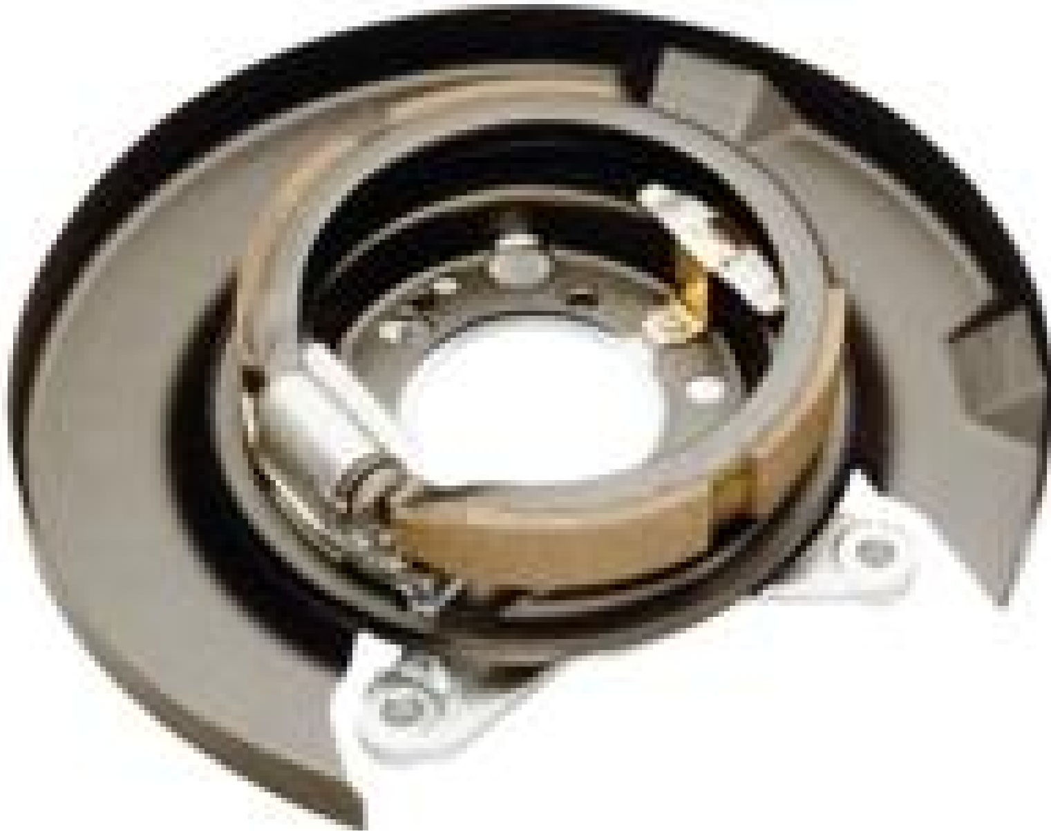
Single-Shoe, Full-Circle Rear Parking Brake with Mechanical Adjuster
