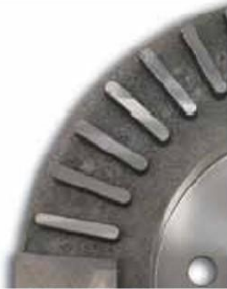
Cutaway view of uni-directional (straight vane) rotor.
